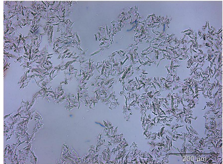
It is likely that the observed viscosity drop in the NFC suspensions during continuous stirring is related to in the structural changes in the suspensions.
