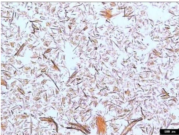
Pulp F - pre-hydrolysis - soda AQ cooking
