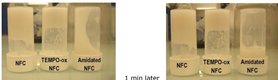
Figure 1 a) after turning and b) 1 min later. NFC produced with mechanical and enzymatic pretreatment before homogenization NFC with tempo oxidation and NFC with tempo oxidation and amidation, consistency 2 %. Gel viscosity decreased after amidation.
