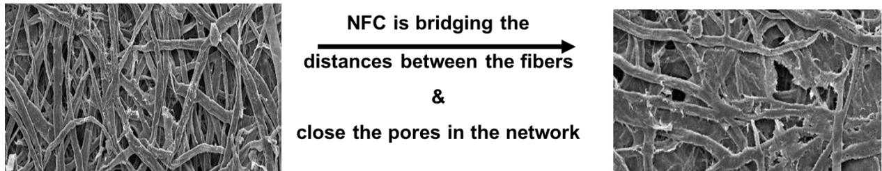
Figure 2 a) and b) Possible applications of NFC in wet end are based on more dense structure or better bonding ability.
