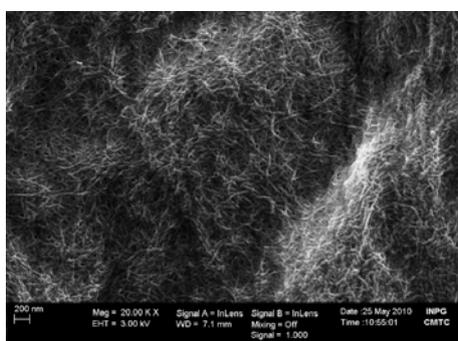
Figure. SEM examination of NFC suspension obtained with enzymatically pre-treated dissolving pulp.
