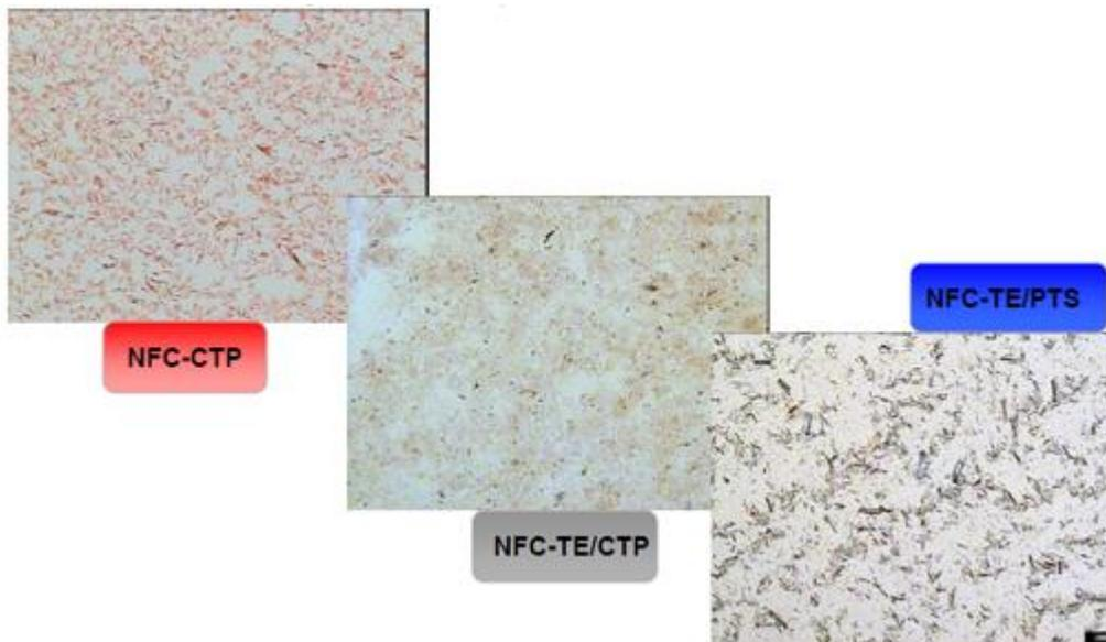
Figure 2. Light microscopy pictures of NFC-CTP, NFC-TE/CTP, and NFC-TE/PTS
