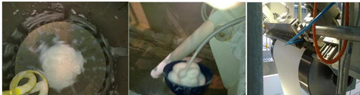
Figure 5. a) NFC in feeding tank (left), b) foamed NFC before application unit (middle), and c) VTT's narrow slot type applicator in a large-scale pilot coating machine (right).
